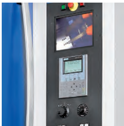
► NC-operator-panel-control with automatic operator guidance ► Optional: camera for grinding area supervision
