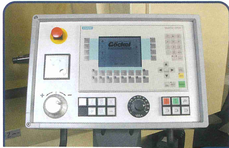
NC-operator-panel-control with automatic operator guidance
