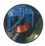
Cup wheel used on press brake dies etc.
